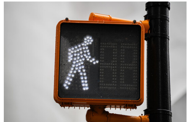
Figure 77: Photo Example of Walk Signal
