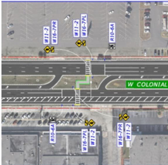
Figure 109: Colonial Drive Proposed Raised Crosswalk at Hyer Avenue
