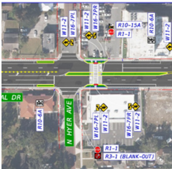
Figure 109: Colonial Drive Proposed Raised Crosswalk at Hyer Avenue
