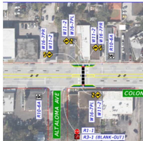
Figure 110: Colonial Drive Proposed Raised Crosswalk at Altaloma Avenue
