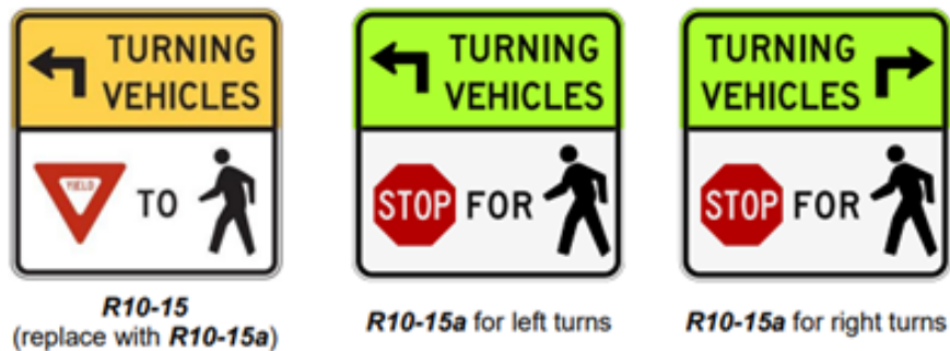
Figure 89: Static R10-15 Turning Vehicles Yield to / Stop for Pedestrian Signage
