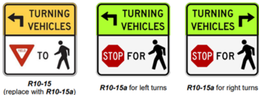
Figure 83: Static R10-15 Turning Vehicles Yield to / Stop for Pedestrian Signage
