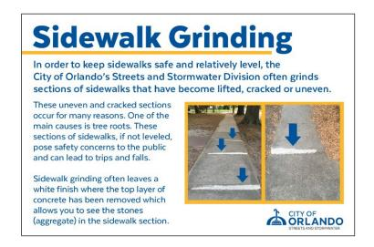
Contractor Crews identified and repaired minor trip hazards through grinding, and when grinding was not an effective solution, crews replaced damaged sections of sidewalk. From 2016 through 2021, contracted crews identified and removed trip hazards and repaired damage at 180,954 sites covering 832 miles of the City's 983 total miles of sidewalk.
