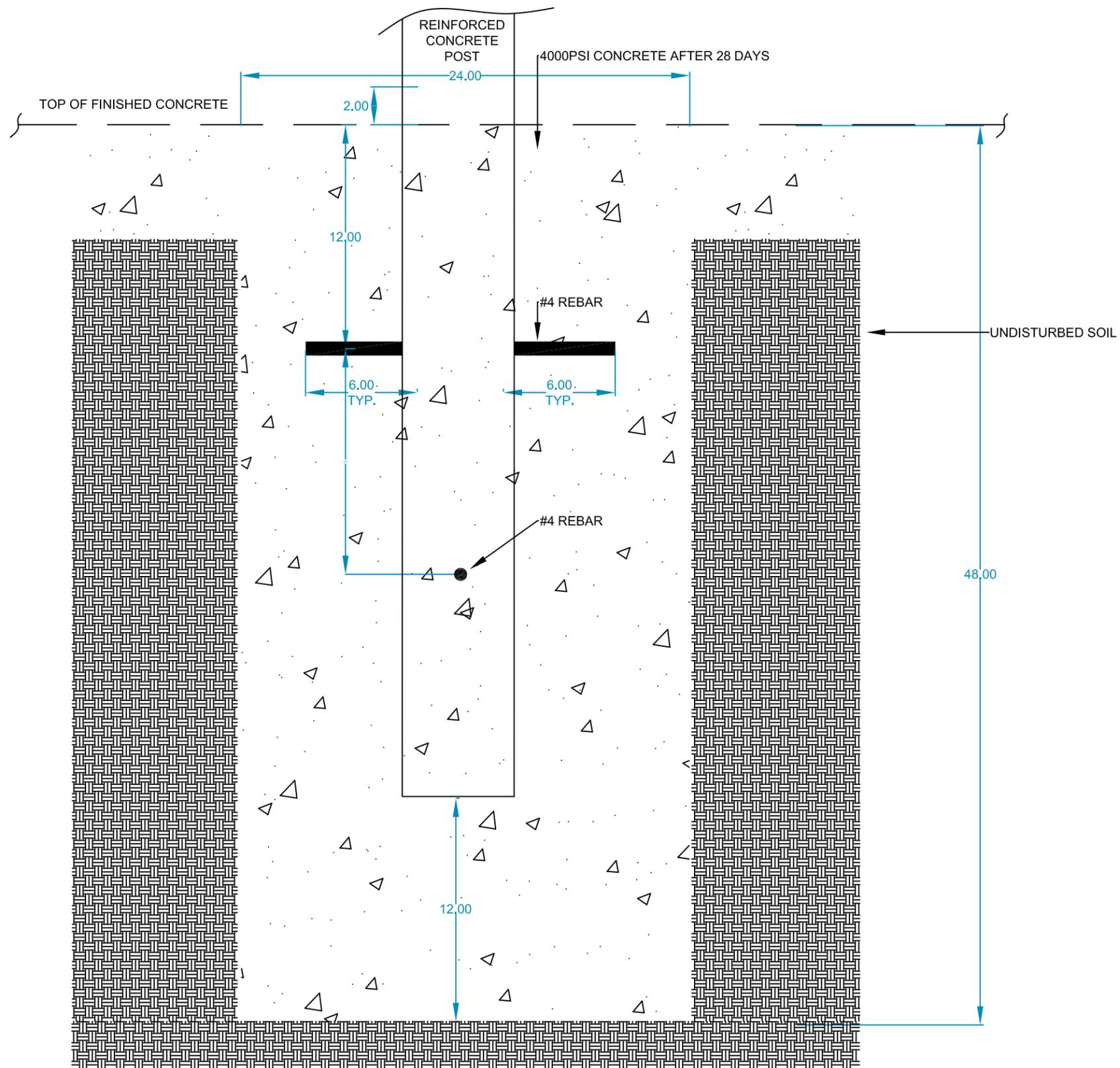
OUTDOOR EQUIPMENT RACK CONCRETE POST BASE DETAIL 1
