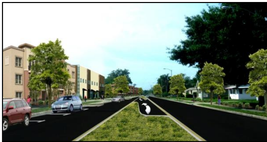
Figure 27: Goldwyn Ave.(looking south) road diet possibilities. This option includes an optional landscaped median.
