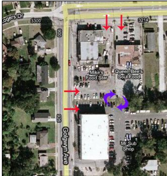
Figure 23: Access management image. Red arrows show existing curb cuts. The purple arrows demonstrate potential cross-access easements.
