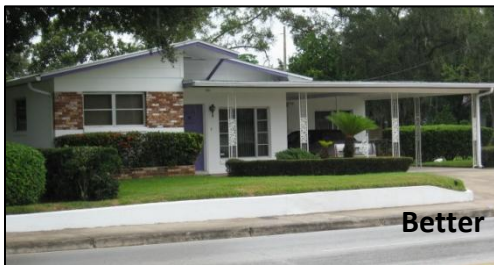
Figure 39: Existing examples of territorial reinforcement. The 1st image lacks clear separation between public and private spaces. The 2nd image uses a knee wall and landscaping to provide that separation.
